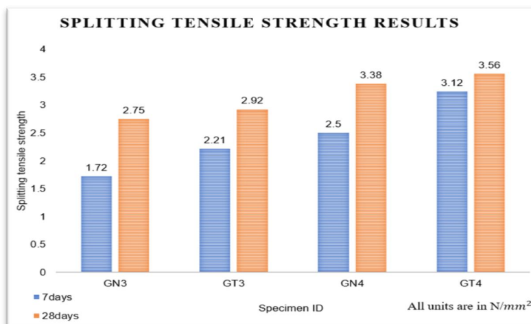
Fig 4 Result of 7 Days and 28 Days Splitting Tensile Strength (Results of Treated water curing)
