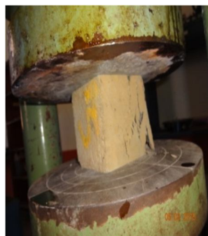
Figure 2 Compressive Strength Test
