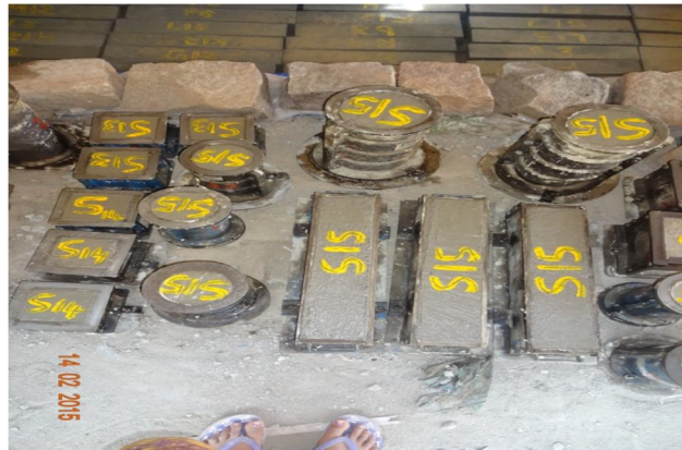
Figure 1 Concrete placed in moulds
