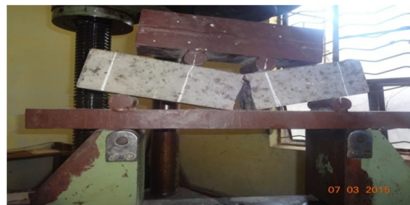
Figure 4 Flexural Strength Test
