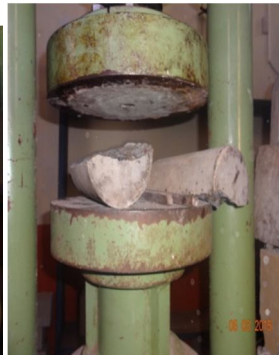
Figures 3 Split Tensile Strength Test
