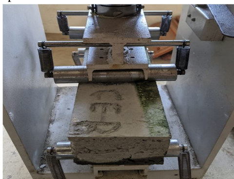
Fig.3. Flexural strength testing
