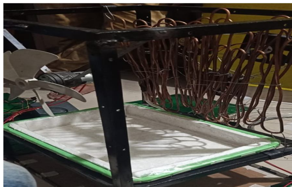
Fig: Piped lining at back with insulated water container
