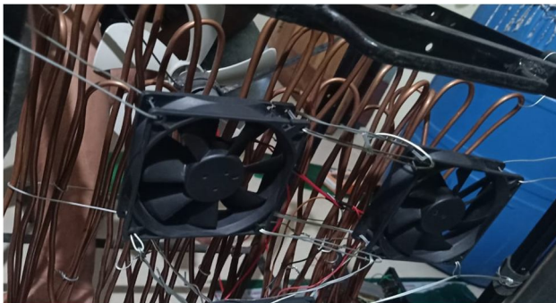
Fig : DC fans for heat dissipation
