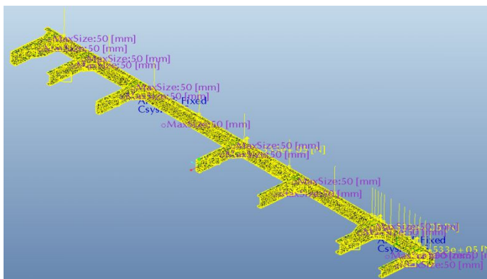
Fig.4 Loading and constraining of Chassis
