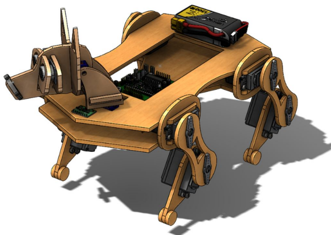
Fig. 1. CANINE: An Autonomous Quadruped Walking Robot
