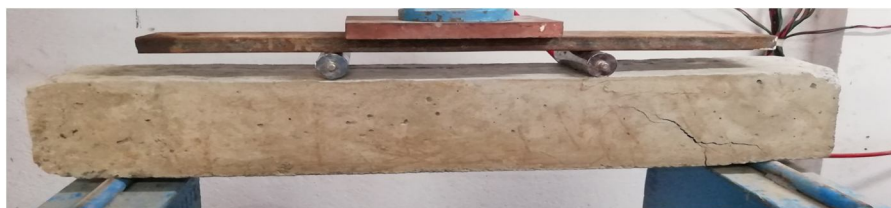
Figure 7 Cracked pattern of geogrid confined beam
