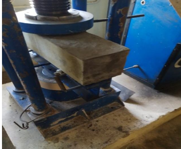
Fig.2 Experimental Setup for Flexural Strength of Beam
