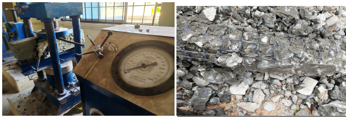
Fig.6 Failure mode of beam during Flexural Strength Test
