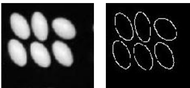
Figure. 5 Segmentation result 1 -Grayscale image, result 2-Edge detection
