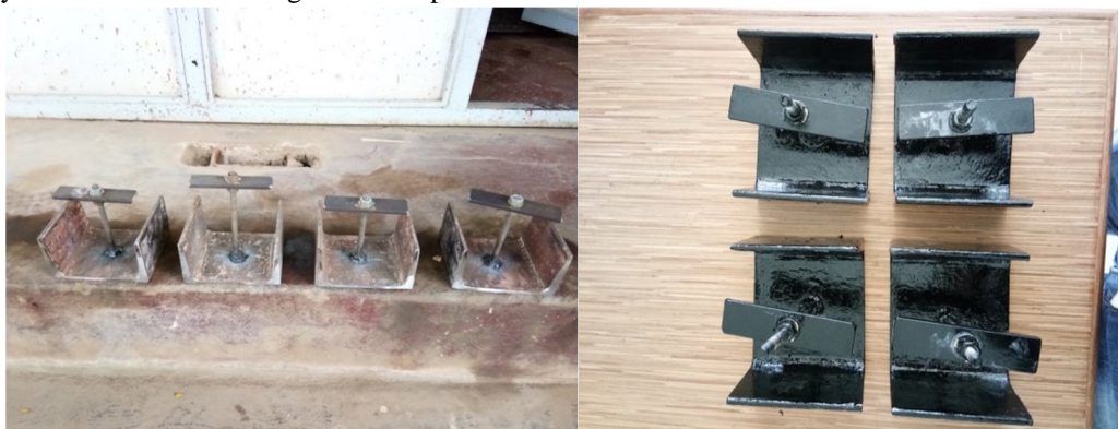
Fig. No.4.1 c-channel preparation
