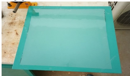
Fig. No.3.11 mylar sheets as mould releasing agent
