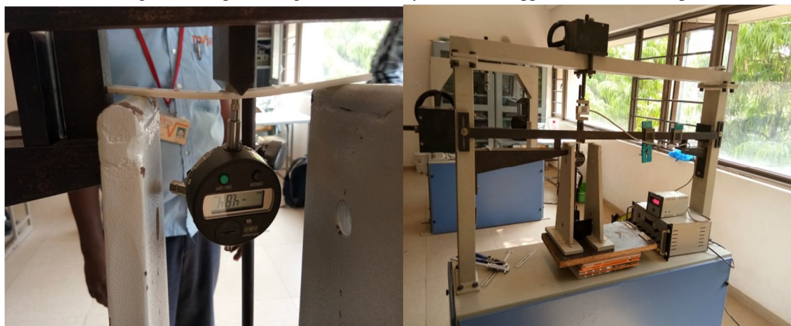
Fig. No.4.3 dial gauge and deflection test
