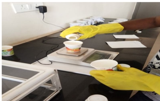
Fig. No.3.9 epoxy ly556 and hardener-hy951 preparation
