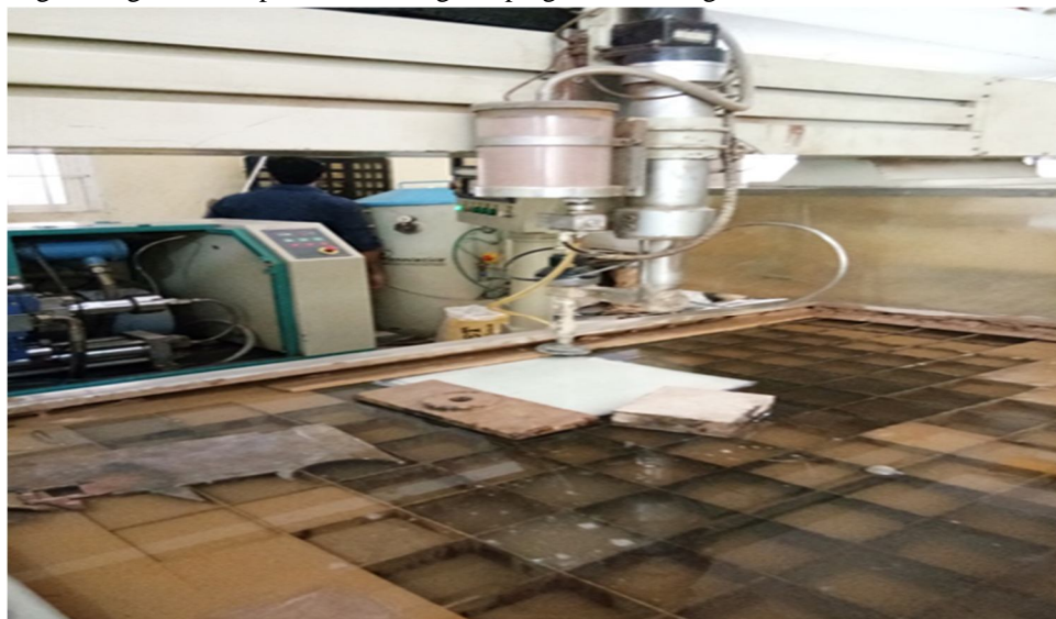
Fig. No.3.18 water jet cutting
