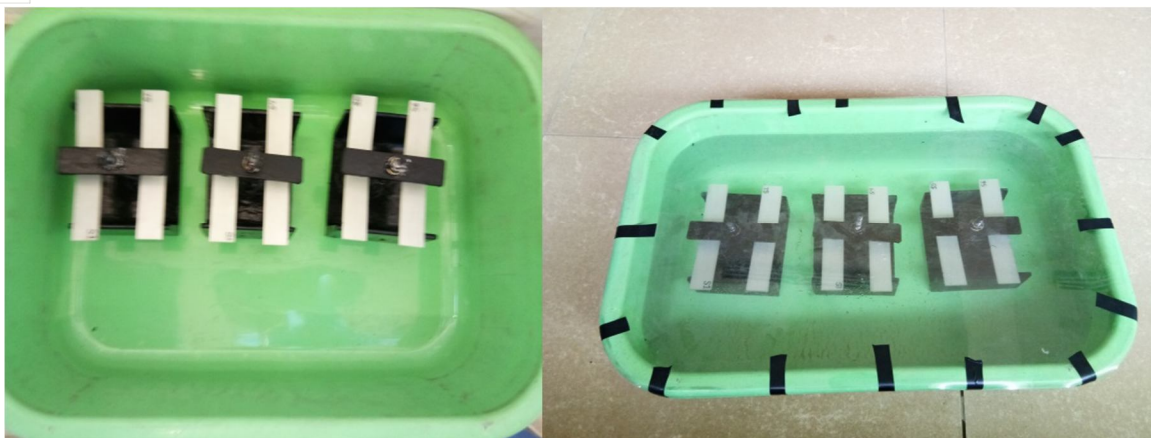
Fig. No.4.4 specimen submerged in sea water
