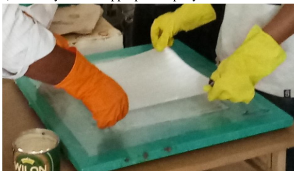
Fig.No.3.13 Placing Of Glass Fabric Over Mylar Sheet
