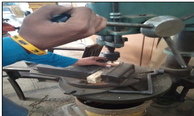
Figure 10. - Drilling procedure of Crankshaft
