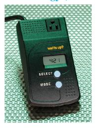
There are several watts up? meter models available. The model that we tested was the watts up? PRO es model which included extra memory for saving measurements that are taken over long periods of time. The watts up? meter has several advantages over the KILL A WATT meter. It has more complex features than the KILL A WATT meter such as more sensitive measurements and memory for data storage.
