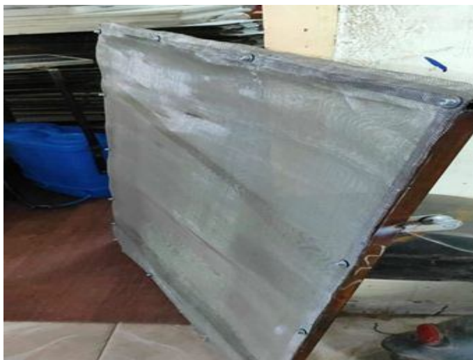
Fig13 : Mesh welded frame
