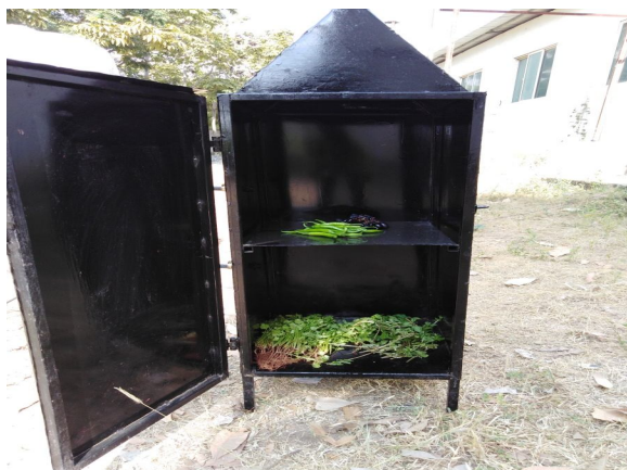
Figure 3.4 Experimental setup of dryer with products
