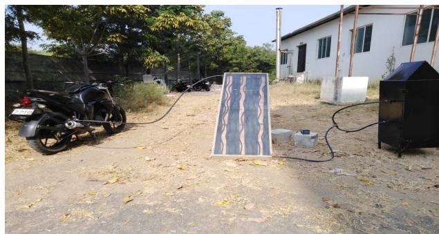
Figure 3.2 Experimental setup by bike exhaust as inlet
