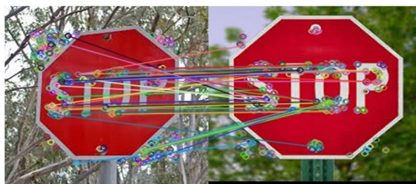
Fig3. (a). Example of Matching in Planar Image Homography
