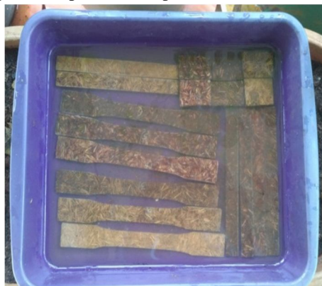
Fig.13(b). Specimens in rain water after 15 days
