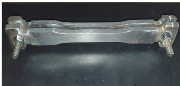
Fig.10. Steel die for Tensile test specimen
