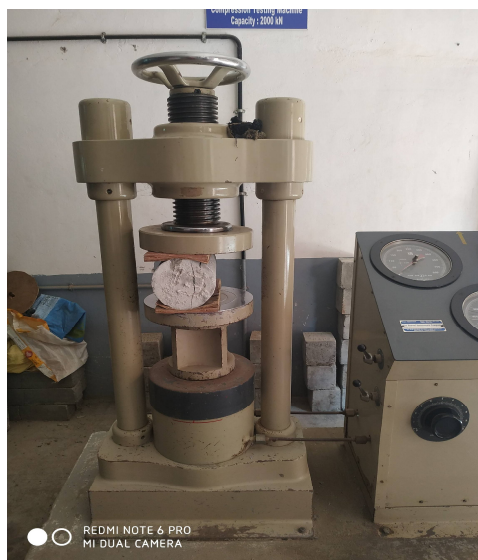
Fig.12 Split Tensile Test on cylinders
