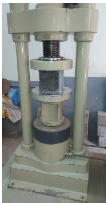
Fig.13 Compression test on cube
