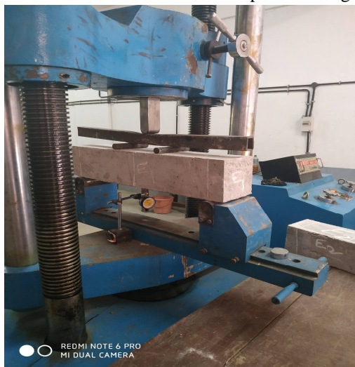
Fig.31 Two point load flexural strength testing method
