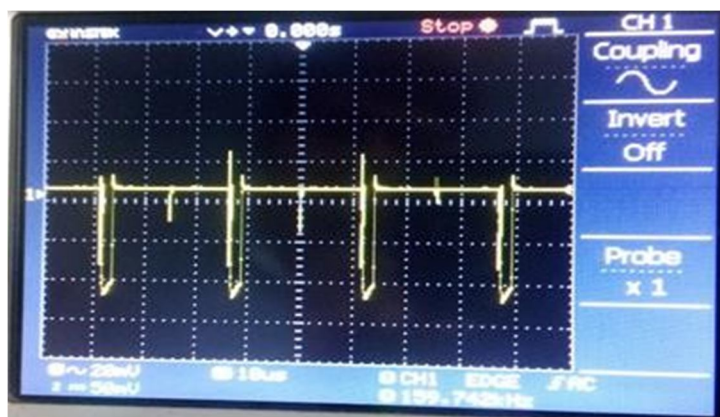
Fig 4.1(viii) Pwm wave in hardware
