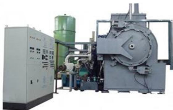
Fig 2.3.2 Heat treatment of specimens on Quenching oil furnace
