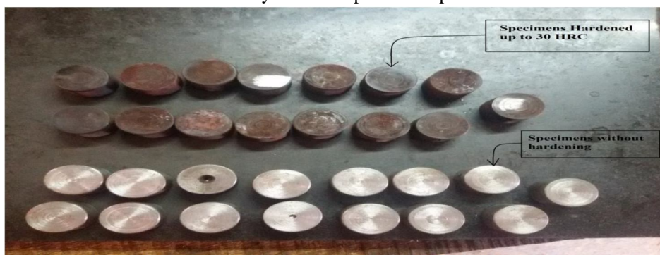
Fig 2.3.4 Specimens ready for machining on CNC
