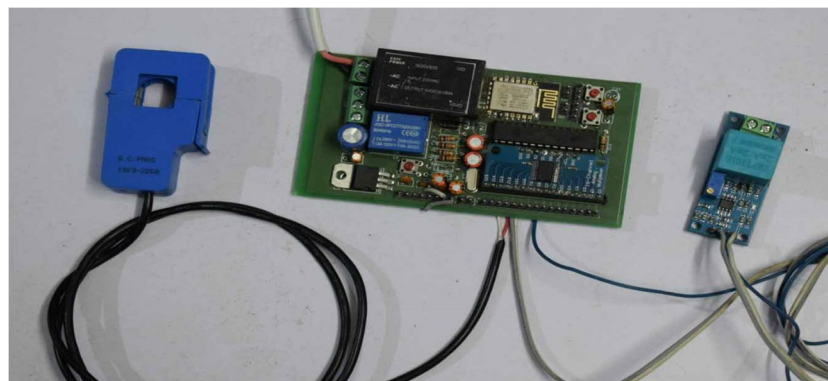
Fig. 7. PCB along with sensors
