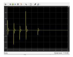
Every suspension system is nonlinear due to its non linear properties spring, damper, and other parts of system. After comparing both graphs it can be clearly shown the nature of graph is nonlinear. But normally for the analysis purposes vehicle suspension spring is assumed to be linear behaviour.
