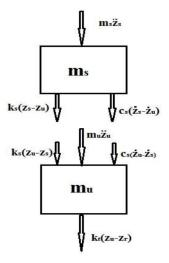
For unsprung mass:  $m_u \ddot{z}_u + k_t (z_u - z_s) - k_s (z_s - z_u) - c_s (\dot{z}_s - \dot{z}_u) = 0$  $\ddot{z}_u = -k_t / m_u (z_u - z_s) - k_s / m_u (z_u - z_s) - c_s / m_u (\dot{z}_u - \dot{z}_s)$
