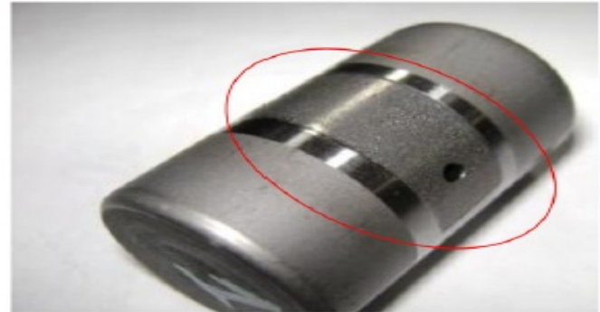
Fig:-1.8 crankpin spalling
