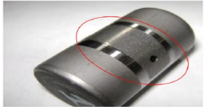
Fig:-1.8 crankpin spalling
