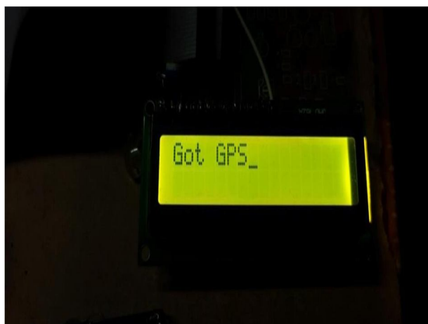
Fig.3.5.The Device got GPS Location when it found Emergency Condition.
