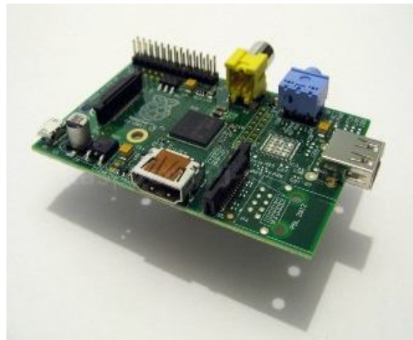
Fig.2. Raspberry Pi Development Board
