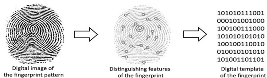
Fig. 1 Bitmap pattern recognition of a fingerprint
