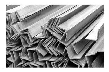
Mild steel can be used for its cost and strength. It is a carbon steel with 0.25% Carbon and 0.4% of manganese, 0.5% Silicon along with some traces of other elements.
