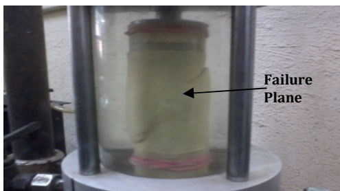
Fig.11 Unconsolidated Undrained (UU) test Samples.
