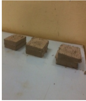
Fig. 6 Failure on Fly ash with 50% PRP
