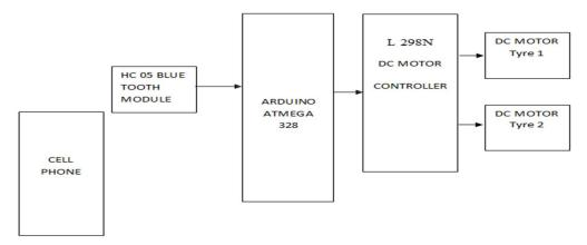
In our project, voice recognition system is used as user interface. The block diagram of the intelligent wheelchair with motor drive and control system
