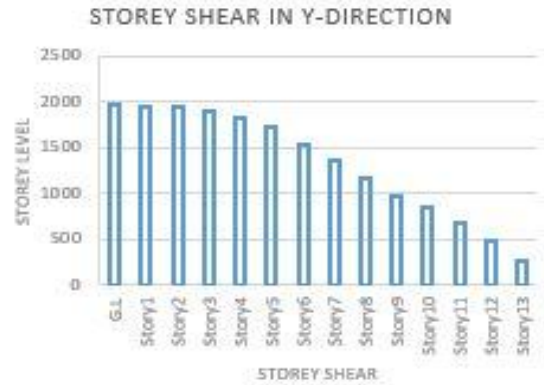
Figure 7.7 Maximum storey shear in direction of Y
