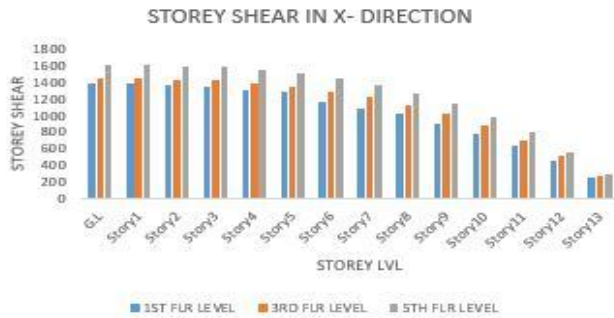
Figure 8.1 Maximum storey shear in direction of X
