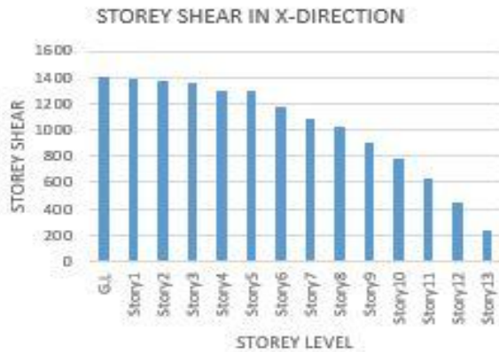
Figure 7.1 Maximum storey shear in direction of X
