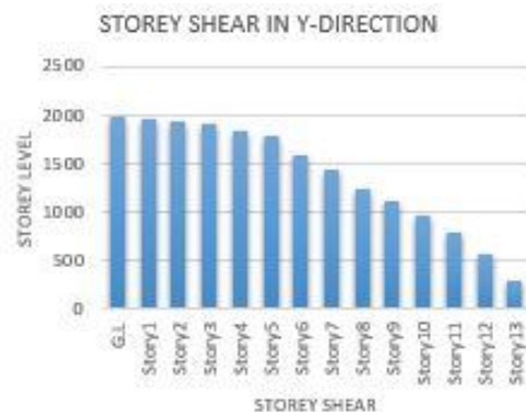
Figure 7.12 Maximum storey shear in direction of Y
