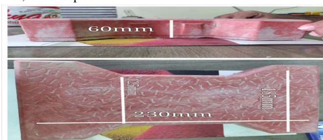
Figure 2: Dimension of Paver Blocks (All Dimensions are in mm)
