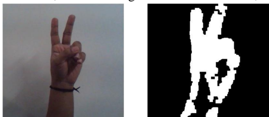
Figure 2: Contour Extraction on detected image
