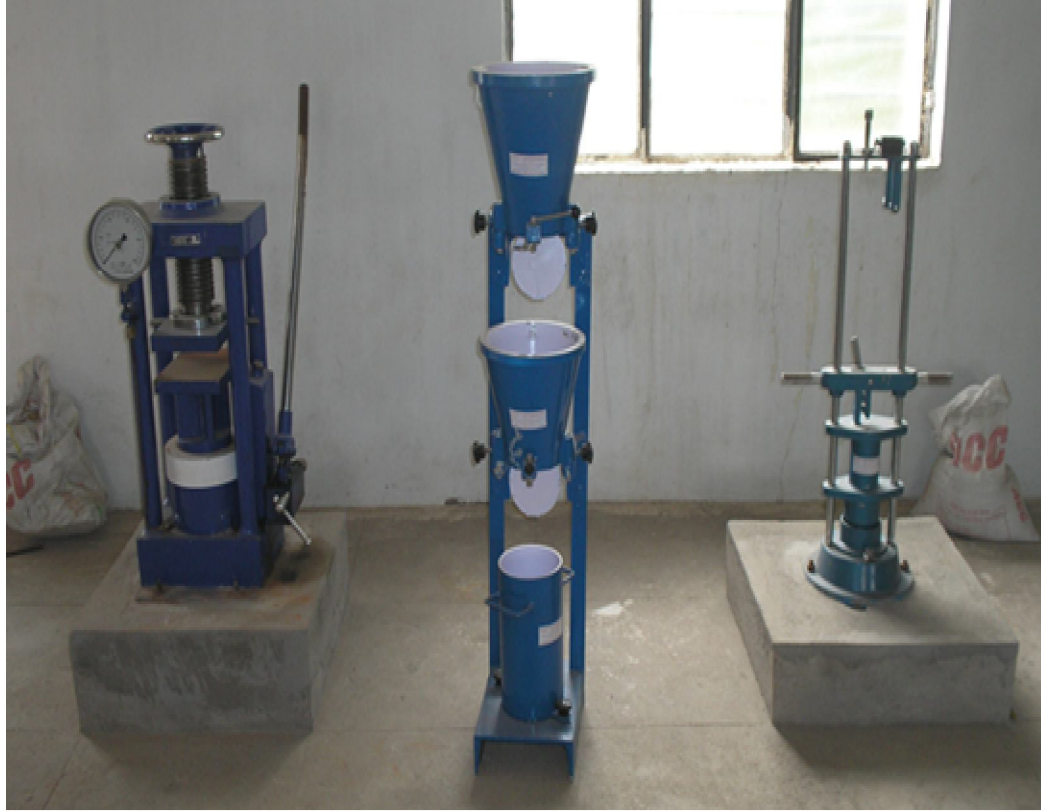
Fig 3.2 Compaction Factor Test
