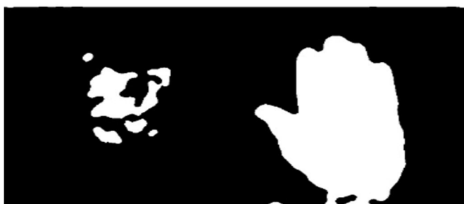
Fig. 10 Detection of the hand eliminating the background
