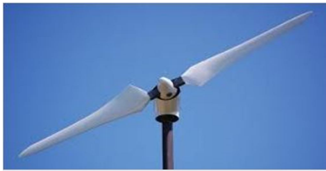
Fig 2.2: Two blade wind turbine
