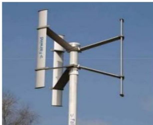
Fig 2.5: H-Darrieus wind turbine
