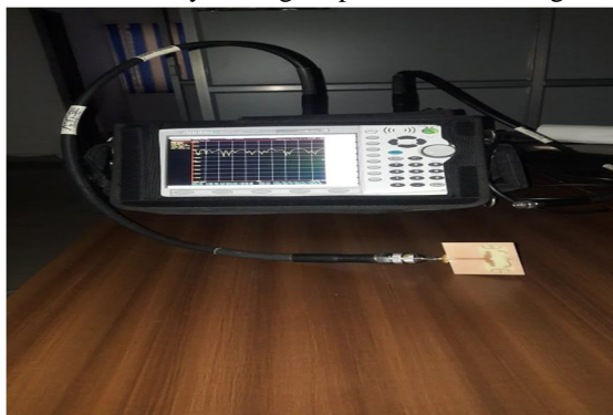
Fig9. Testing in Vector network analyzer
