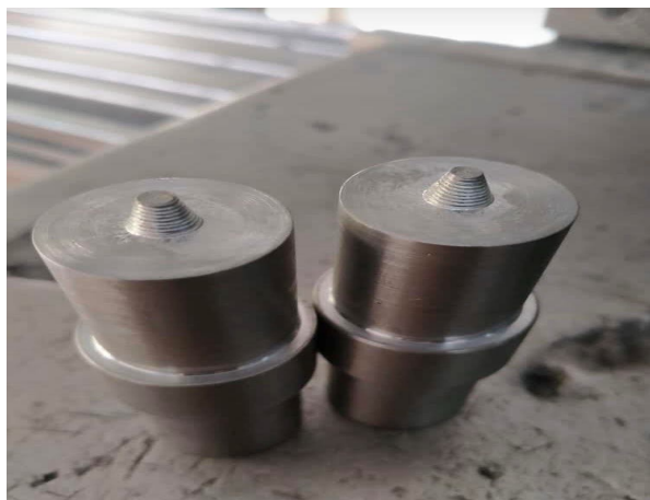
Figure 2: A taper cylindrical tool profile
