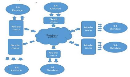
Show in Block Diagram Raspberry pi work as a hub and multiple node MCU connected to the Raspberry Pi. Each node MCU interface with 14 Device.
