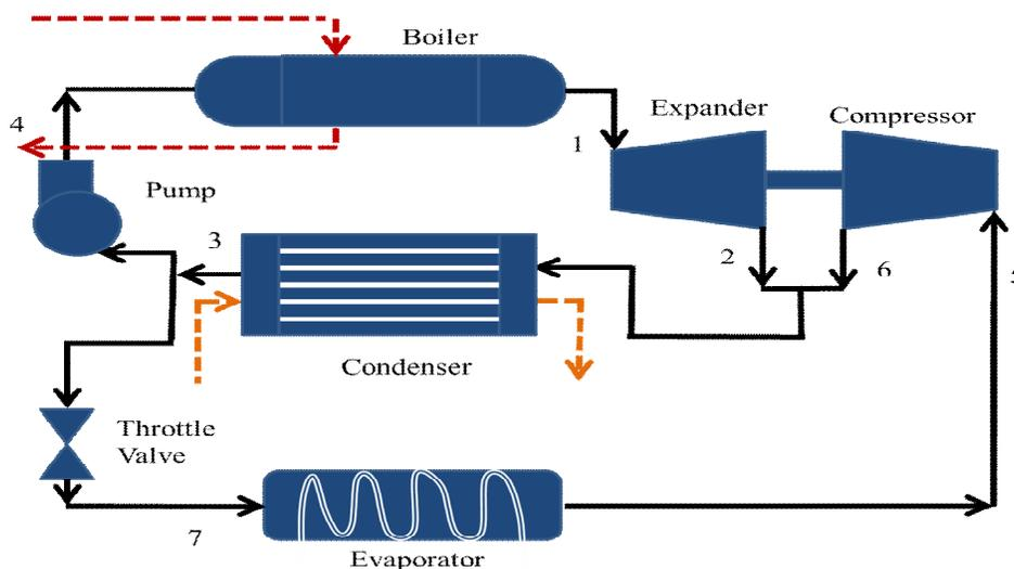
Fig. 2. Schematic diagram of the Combined ORC-VCR system
