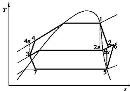
Fig. 3. T-s diagram of the combined ORC-VCR system
