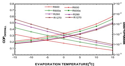
Fig. 8. Variation of COP<sub>overall</sub> and MKW with evaporation temperature
