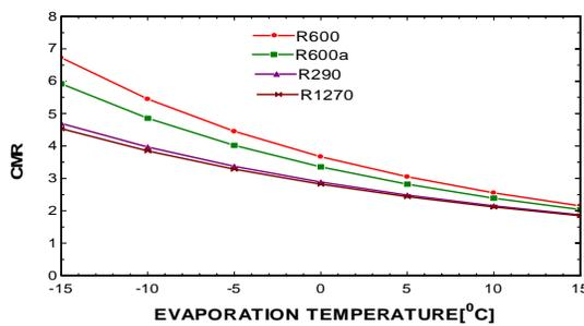
Fig. 9. Variation of CMR with evaporation temperature
