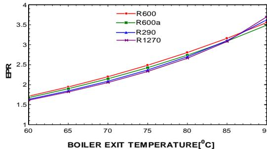
Fig. 5. Variation of  $EPR$  with boiler exit temperature.
