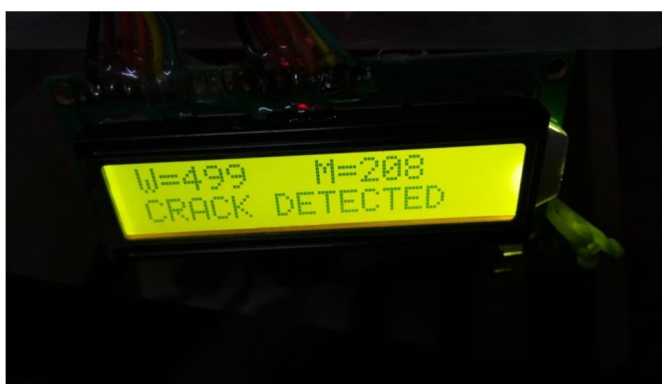
Fig. 10. LCD shows the message crack detected.
