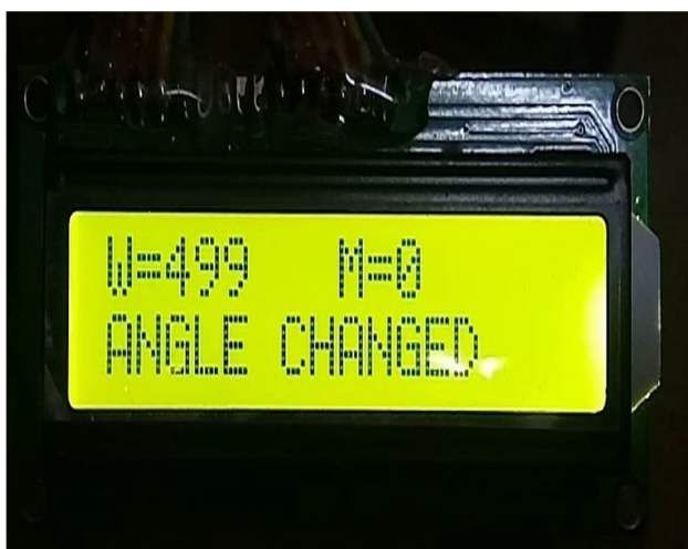
Fig. 7. LCD shows the message angle changed.
