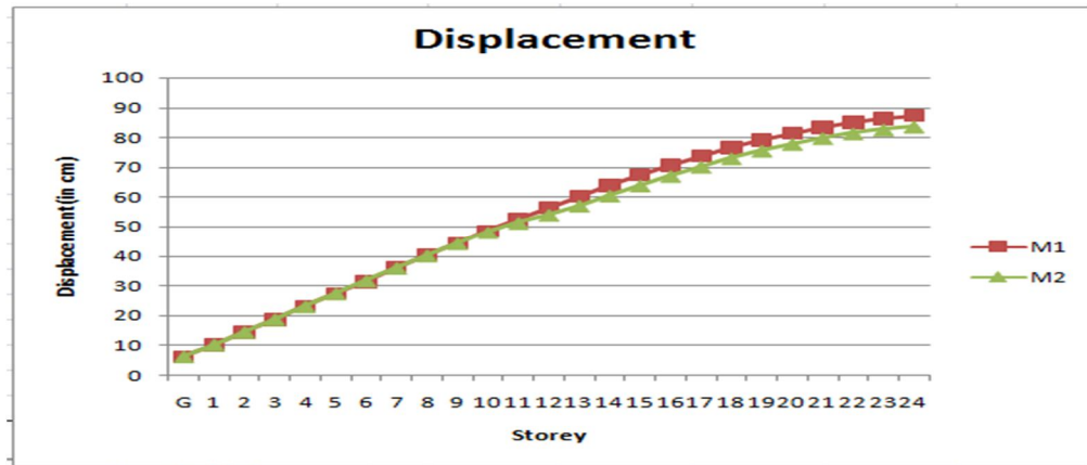
Fig. I Comparison of displacement in X direction of models M1 and M2 for case2
