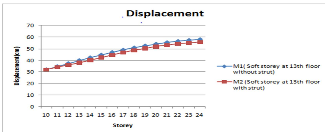
Fig. F Comparison of displacement in X direction of models M1 and M2
