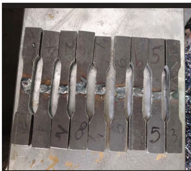
Figure 3: Dimensions of tensile specimen prepared as per ASTM: B557M-10 guideline
