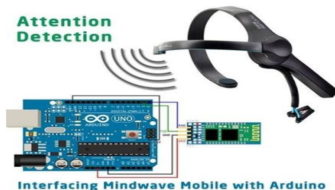
Fig. 4. Neurosky Mind Wave Headset
