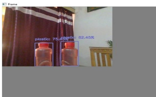
Fig-10 Two Plastic Objects Detection using Caffe Model
