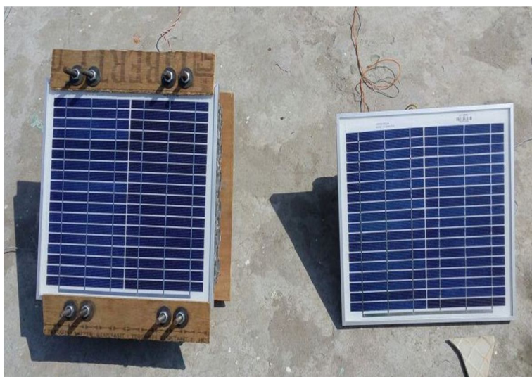
Fig:5 Experimental setup(PV panel with & without cooling)
