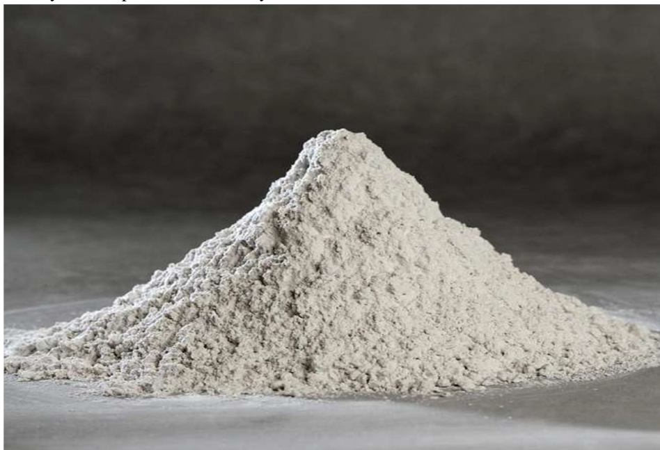
Fig 2: Ground granulated blast furnace slag
