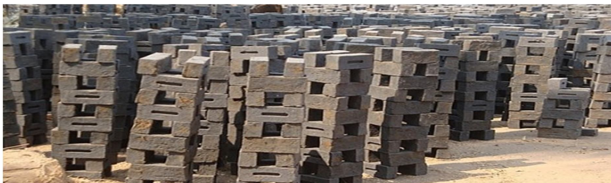
Fig 5: Rice husk ash bricks
