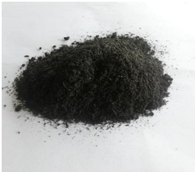
Fig 4: Palm oil fuel ash
