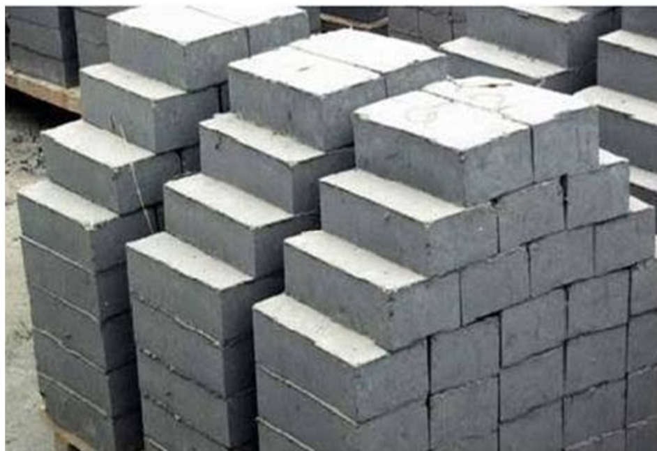
Fig 1: Fly ash bricks
