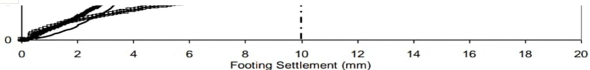
Figure 3: Load-Settlement graph of Test 1 – Half Length Columns
