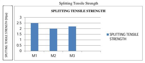
The test results confirm the decrease in the split tensile strength for M2 and M3 mixes.
