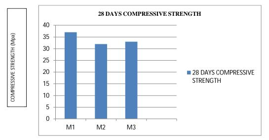
From the test results its is found that there is decrease in compressive strength of M2 mix by 18.51 % and 15.08% for 7 and 28 days respectively when compared to the control mix M1.
