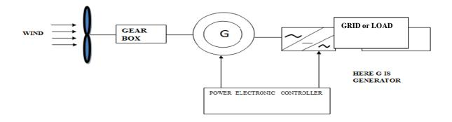
The energy from wind can be harnessed with the help of wind energy conversion system. The aeroturbine converts the energy in wind into mechanical energy first. Then fine tuning with proper pitch control is required. A mechanical gear system of step up type www.ijraset.com Volume 3 Issue VIII, August 2015 IC Value: 13.98 ISSN: 2321-9653
