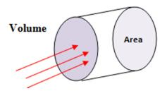
So, mass flux =  $\rho$  x **A** x **v**. The kinetic energy per unit time provides power. Here A is the area swept by the rotor.
