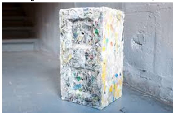
Fig 2- Brick specimen made up of waste plastic. (Source:- www.expertskiphire.co.uk )
