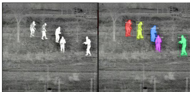
Figure 4: Detection of an abnormal object in an image; (a) Input image (b) Output image
